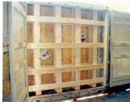
72 Steel Drums secured with a AAR approved wooden gate
