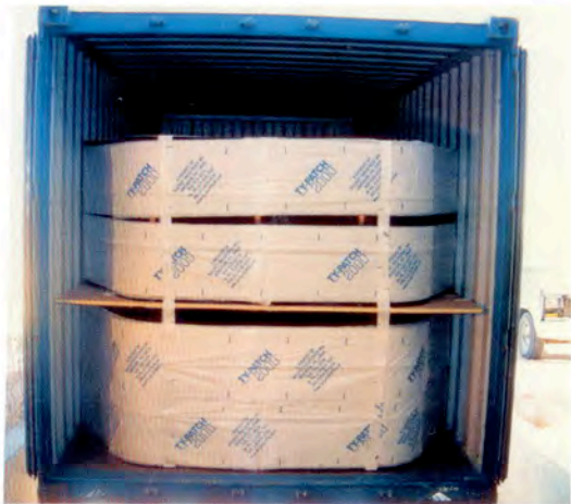
78 Steel Drums secured with Ty-Gard 2000®
